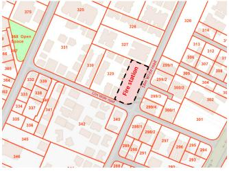
Figure 57: Locating Fire Station on narrow road shall be avoided.
