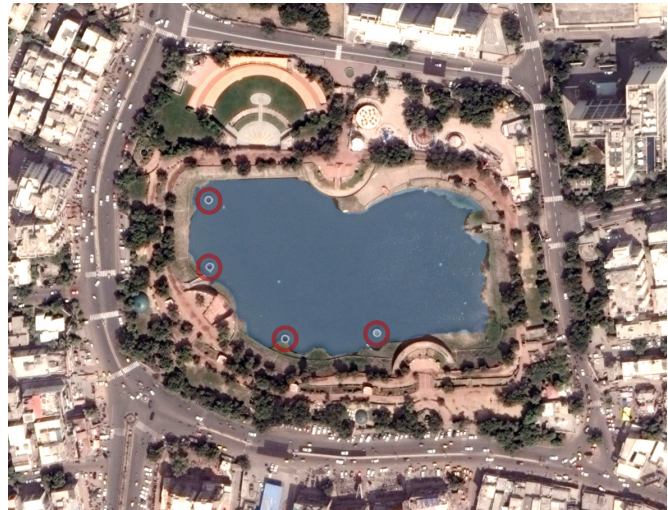
Figure 7_32: Networking storm water drains to rain water recharge wells in Vastrapur lake- a case of good practice source: Google Earth Satellite Image
