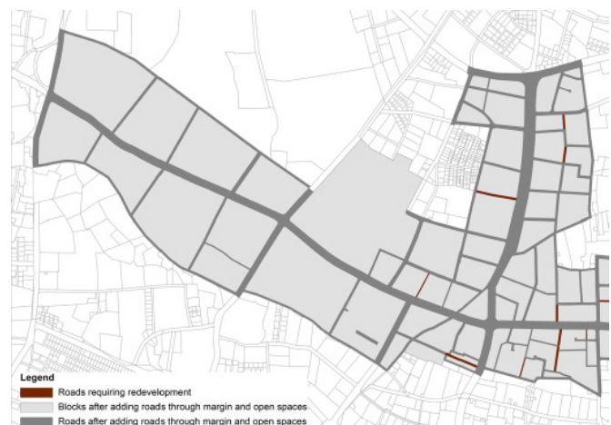
Step 5: Adding new roads requiring Redevelopment
