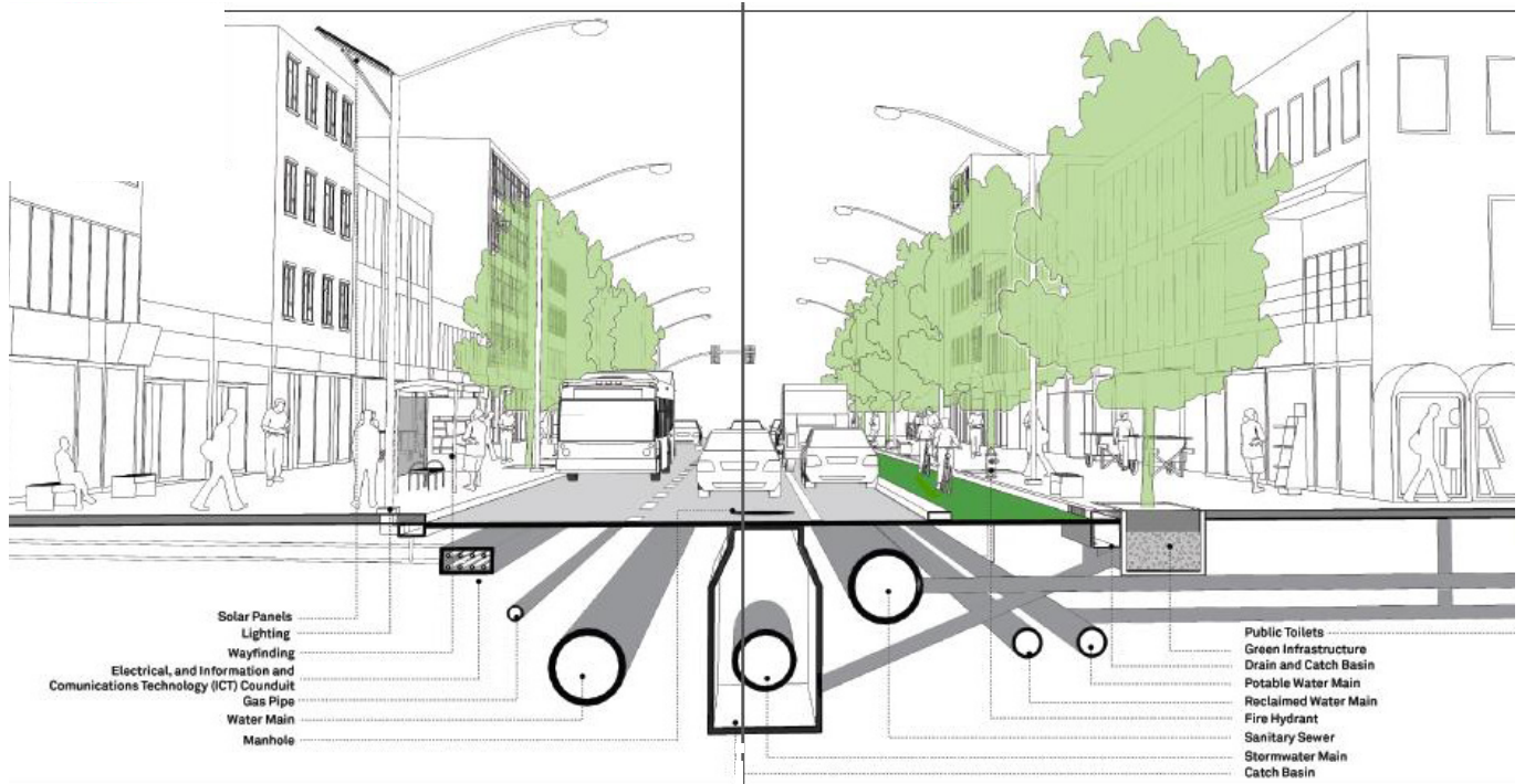
Figure 7_31: Provision of Underground Utilities based on the street type and context Source: Global Street Design Guide, NATCO
